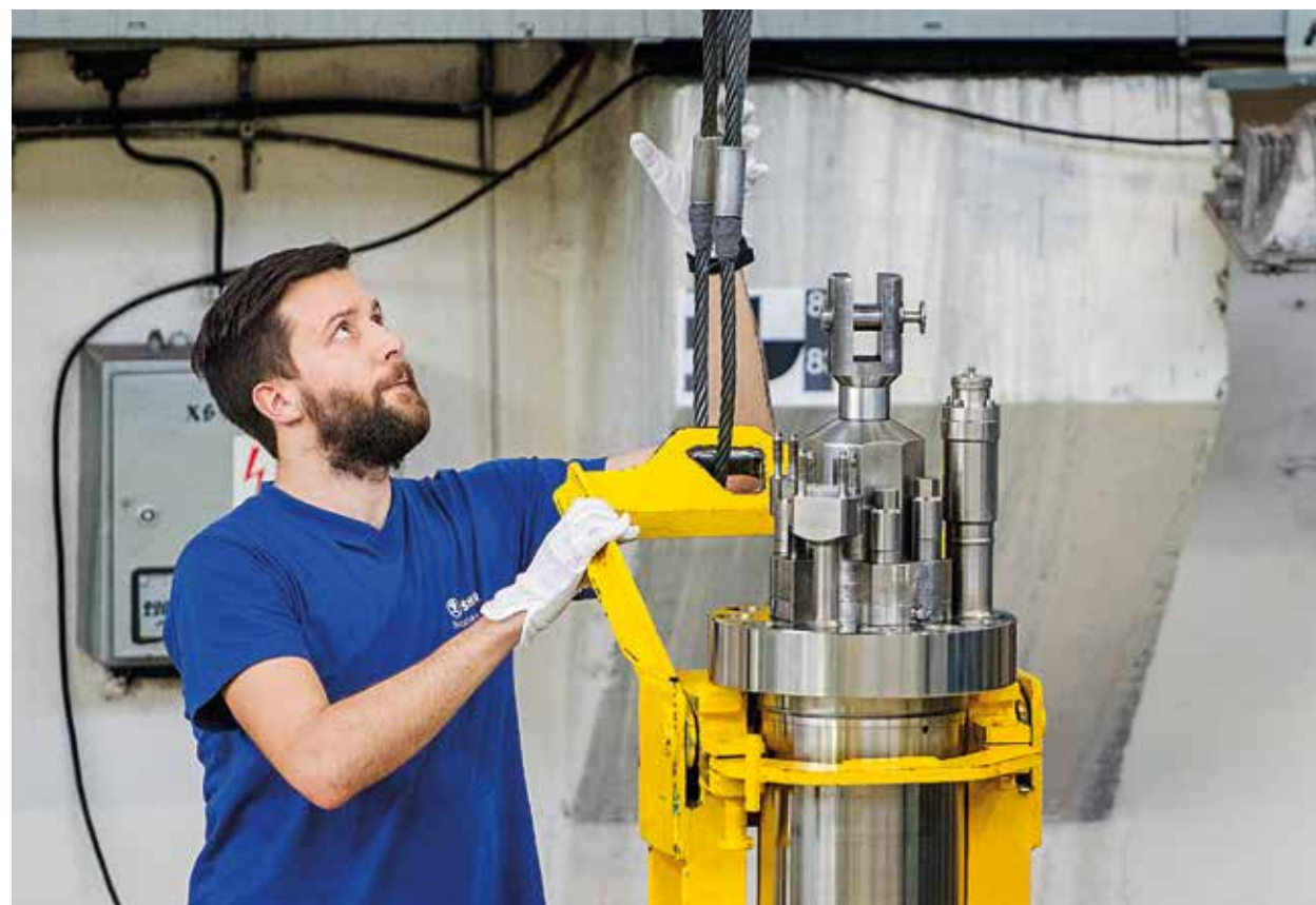
Handover tests of new PRO-M drives for the Bohunice and Mochovce NPPs, performed on the "Large Water Loop" stand (LWL).
