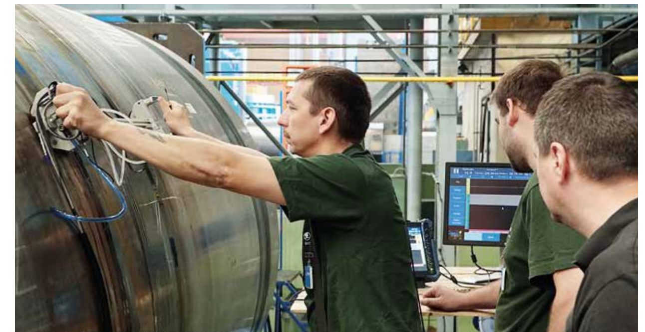
Ultrasonic testing of a ŠKODA 1000/19 cask weld by a newly acquired and introduced TOFD method
