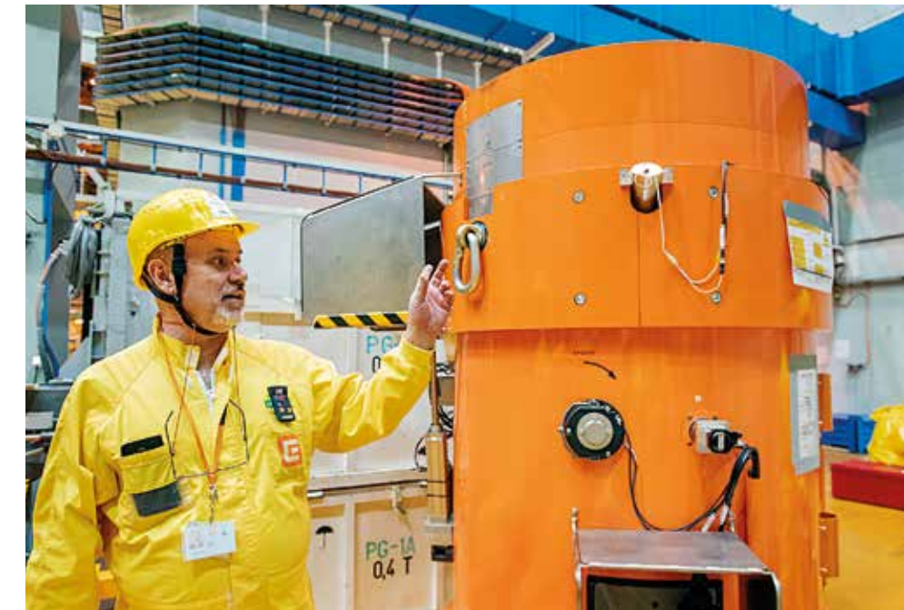
The device for removal, transport and disposal of VVER 1000 reactor thermocouples and neutron flux sensors, developed and manufactured by ŠKODA JS.
